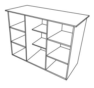
3. Insert horizontal dividers evenly spaced as shown, secure with brad nails
