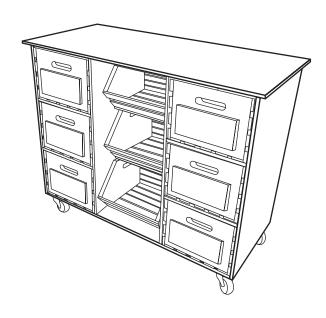
4. Insert crates and secure casters to base using wood screws
