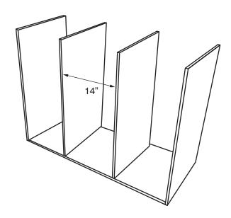
1. Arrange vertical plywood boards (the middle dividers 14" apart) and secure through base with brad nails
