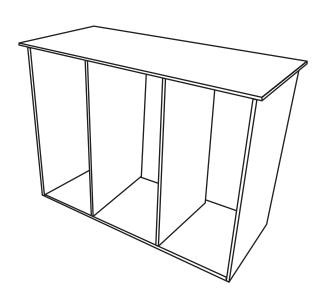
2. Attach top so that there is an even overhang on all sides and secure with brad nails
